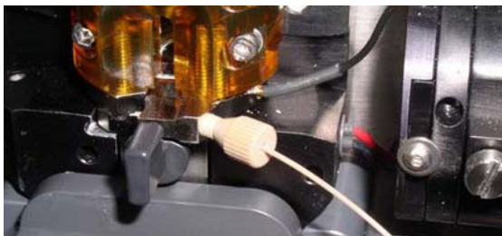
Figure 6-1 Closed-loop nozzle installed in flow cell
